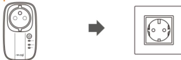
The power of Smart Plug will be on and wait till the Wi-Fi LED flashes quickly.
